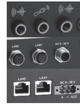
Optional I/O ports for audio, LAN jack type and DC-in jack type
